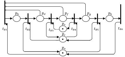
mentioned firing rule and simultaneously if the input places linked to the transition by inhibitor arcs have no tokens. The relevant solution is shown in Fig. 10.
