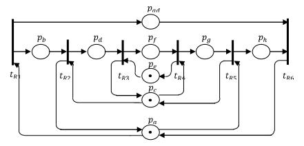
Fig. 9 Modified Petri net model of deadlock-free control procedure.
