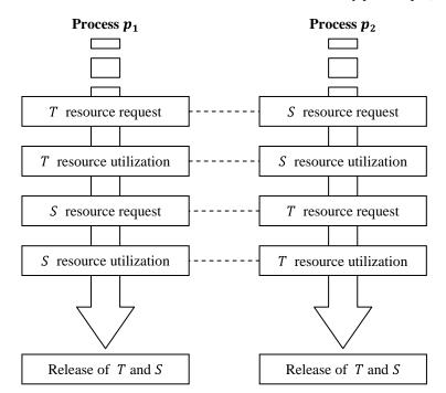
Fig. 3. An example of two processes cooperation while accessing the critical section containing two resources T and S.
